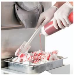
To better variegate gelato in the tray, the beater speed can be reduced, even stopping extraction completely allowing the easy distribution of toppings. Then, increasing beater speed again, extraction continues.
