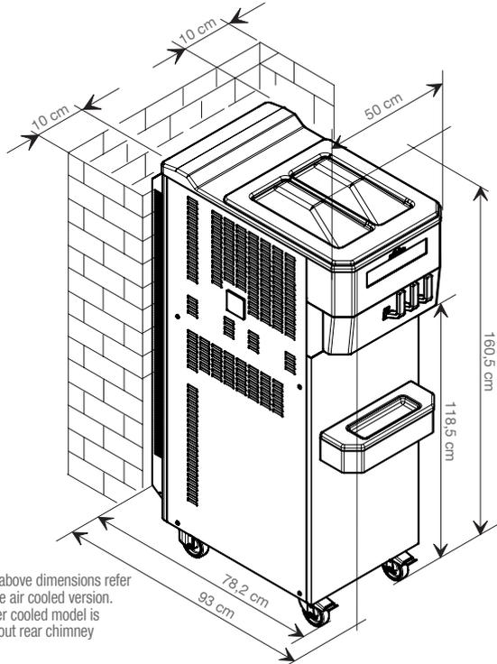
The above dimensions refer to the air cooled version. Water cooled model is without rear chimney
